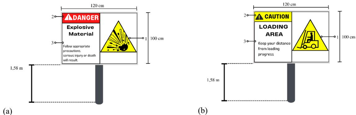
**Figure 9 – (a) Dimensions of explosive material signs (b) Dimensions of loading progress signs**
